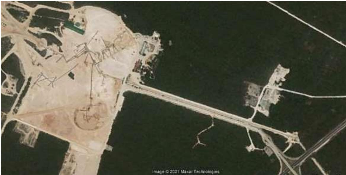
Figure 9. Details of the staging area, conveyer bridges, offices, fuel storage, and roads and large conveyer bridge.
